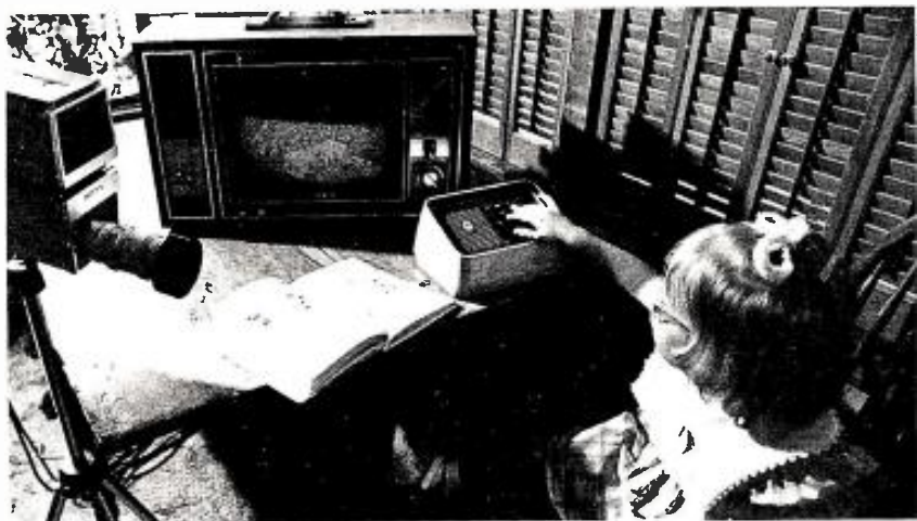
This mock-up shows how the two-way communication system to be tested next month by Telecable Co. will be used for the instruction of disabled children in their homes. The child's hand is on the terminal, which she would punch in a predetermined sequence to get the teacher's attention. After the teacher also punches the terminal at the other end the two can talk to each other. Cameras at both ends permit them to see each other and to display artwork, graphs or other visual material.
