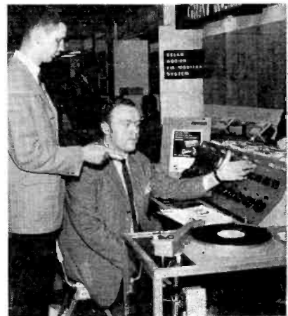
The T-40 action console with four built-in cartridge players from SIS Electronics is shown by its designer, Jim Blanchard (l), to David Calef, director of broadcast operations, WKVT Brattleboro, Vt.
