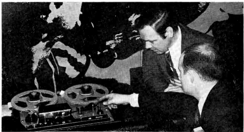
Scully 280, tape recorder, featuring disk brakes and selective synchronization, is shown by representative Mike Faulkner
