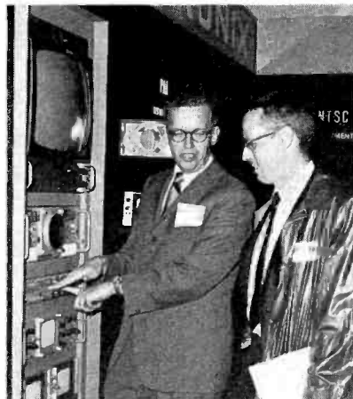
Art Anderson (l) of Textronix explains to Dick Walters, marketing manager for Scientific-Atlanta, Atlanta engineering firm, this year's improvements and how to use the Type 140 test signal generator.
