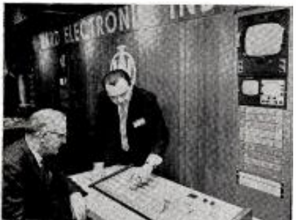
L. E. McBride (seated), CKCK-TV Regina, Sask., listens as Gil Jaeger of Ward Electronics Industries tells how double re-entry switches help make Ward's Type TS-206 console and switching system more effective.
