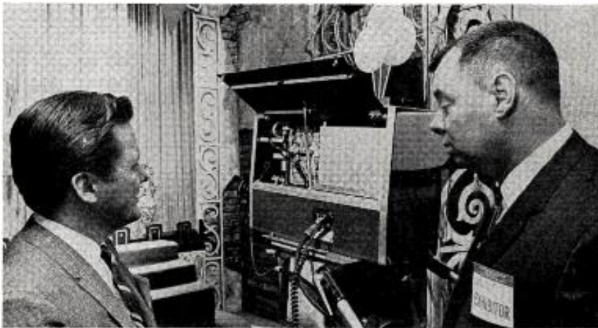
Ampex Corp's new lightweight two-tube BC-200 color camera (above) is opened up by John Reinke for benefit of Thomas Keller, chief engineer of WGBH-TV Boston. The BC-200 is a studio version of hand-held BC-100 that was also featured at this year's show.
