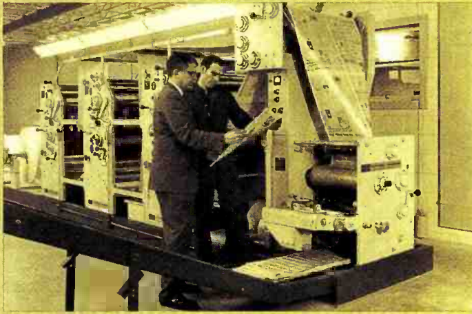
In newspaper publishing by web offset. . . the Cartersville, Georgia, Daily Tribune News , circulation 5,000, and its weekly counterpart, the 3,600-copy Tribune News , have switched to offset with the installation of this three-unit Cottrell Vanguard web offset newspaper press. Shown with the new press are Tribune president John T. Fleetwood and a pressroom employee.
