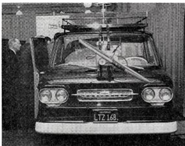
The rotating hoop in the front of truck (l) is the key to the television set counting conducted by Tanner Electronic Survey Tabulations. The hoop receives signals from the sets and matches them through a 'comparator' in the truck to signals from the stations. The station signals are picked up through the antennas on the truck
