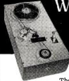
The new Model TP-1A is a rugged, dependable and field tested unit. It is easy to operate and fills a need in every station using cartridge equipment. Will handle all reel sizes. High speed winding at 22 1/2" per second. Worn tape in old cartridges is easy to replace. New or old cartridges may be wound to any length. Tape Timer with minute and second calibration optional and extra. Installed on winder or available as accessory. TP-1A is \$94.50, with Tape Timer \$119.50.
