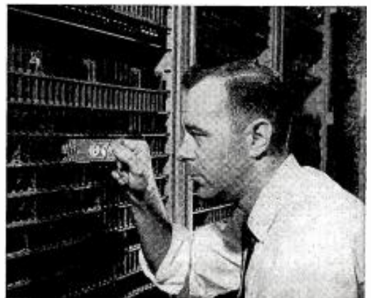
PLUG-IN PACKAGE made by Western Electric for Electronic Central Office consists of transistors, diodes, and other electronic components. Thousands of these cost-cutting printed circuit boards were used.
