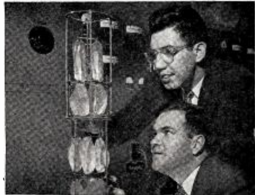
STUDYING QUARTZ CRYSTALS "grown" synthetically for Bell System communications equipment at Western's Merrimack Valley Works in North Andover, Mass., are R. A. Laudise (at top) of Bell Telephone Laboratories and R. A. Sullivan of W. E.
