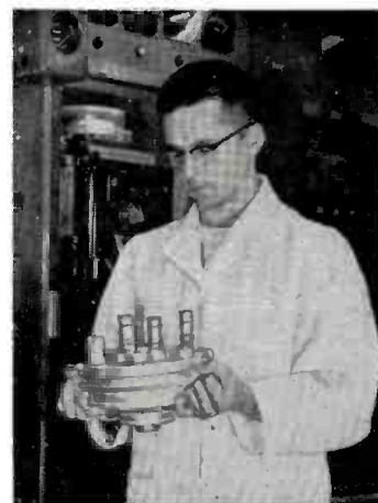
Compact, lightweight, and easy to handle, RCA-6806 delivers 28 kw TV output at 550 Mc.
