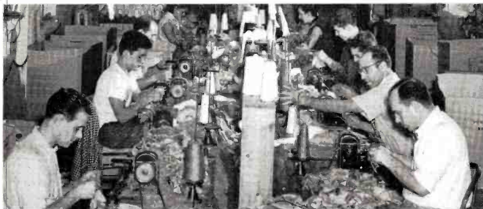
THE SEWING ROOM , where the jigsaw of cut-out parts starts to take shape. After the face—made of pliable vinyl plastic—is sewn on, the doll is given a cotton stuffing via a pneumatic machine, and wires are inserted in the legs to enable the dog to stand.
