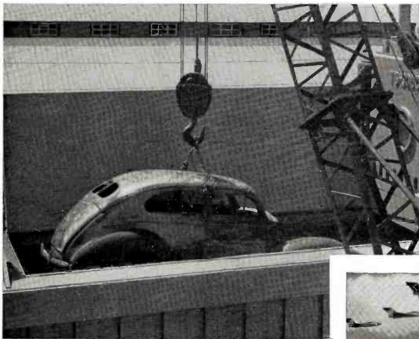
It Goes In There. This junkyard baling press gobbles up two cars or one truck at a time, and squeezes them into a tight bale of scrap steel.
