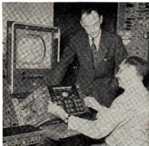
A. R. HOPKINS (seated), manager of RCA Broadcast Equipment Marketing, and Theodore A. Smith, vice president-general manager of RCA Engineering Products Div., demonstrate how the newly-developed color processing amplifier's compact design permits its mounting in a section of a control room console.
