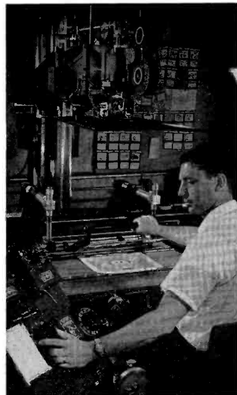
TRANSFILM's specially-designed animation camera stand in use.
