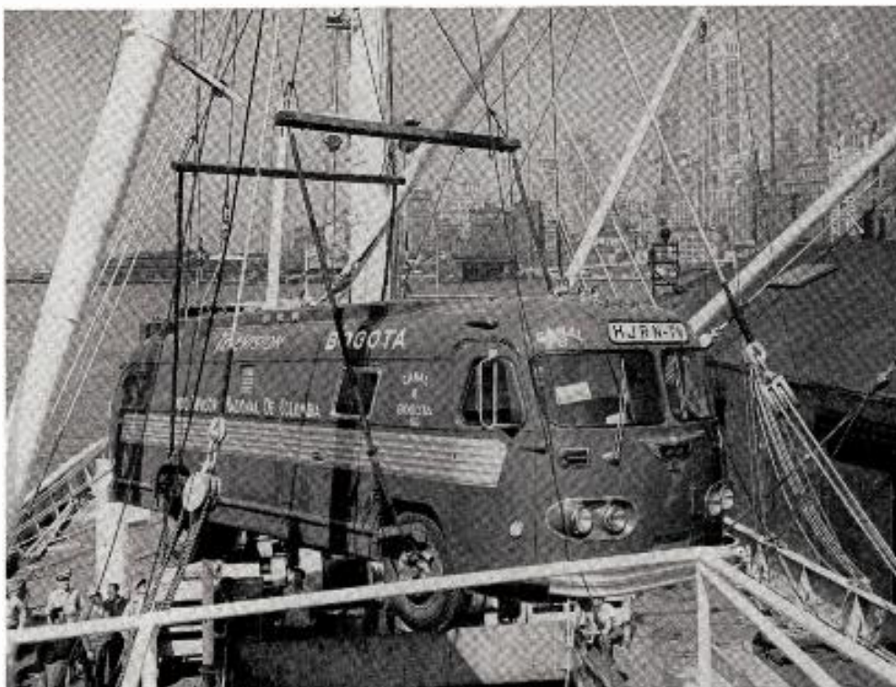
A DuMONT TELECRUISER, mobile tv station for remote pickups, is lowered into the hold of the Ciudad de Quito on its way to HJRN-TV Bogota, Columbia, the first tv station in that country. The Telecruiser was completely designed and equipped by Allen B. DuMont Labs and built by the Flexible Corp. of Loudonville, Ohio.
