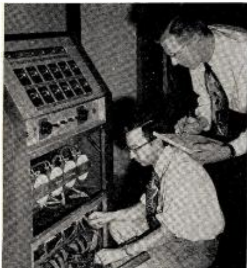
RCA's first 50-kw vhf tv transmitter gets final test and inspection at the company's plant at Camden, N. J. The transmitter has been shipped to Minneapolis to be used by ch. 11 sharetimers WMIN-TV and WTCN-TV [AT DEADLINE, Feb. 15].
