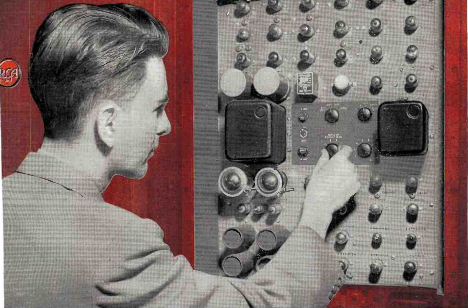
New RCA single-unit Sync Generator takes less than one-third the rack space needed by other sync systems
