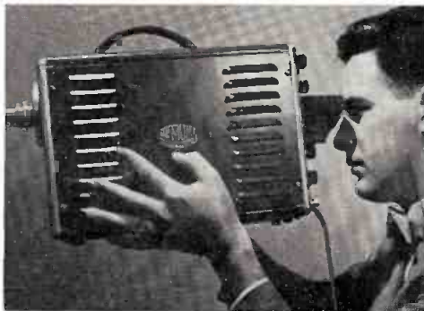
AN 18-POUND portable TV camera designed to replace a standard 350-lb. setup was shown by Allen B. DuMont Labs. at the IRE convention. Called the Tel-Eye, the camera will plug into a standard wall socket. It is 14 in. long, 9¾ in. high and 4⅝ in. wide. DuMont sets the price at $2,850.
