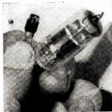
LEFT to right are the germanium core of a transistor, the transistor itself and the subminiature tube the transistor replaces.
