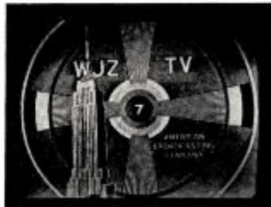
TEST pattern of WJZ-TV New York before (l) and after (r) Aug. 9 power boost from 3 kw to 16.3 kw. Both pictures show reception on "an average" television set in the so-called "fringe" area.
