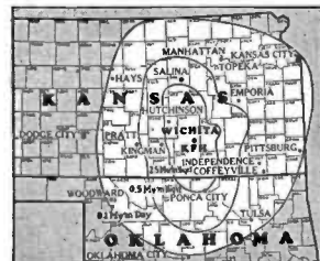
Class D. Cities Compared Field Strength Distribution Based on Performance and Terrain Survey Measurements—5000 Watts Day and Night—October 1941
