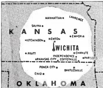
Green: D. Gullett Field Strength Survey—1939 Map Shows Coverage to the .1 MV/M Line
