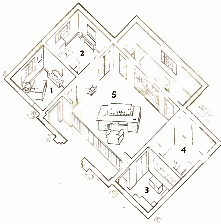
NEW TRANSMITTER LAYOUT—Here is the floor plan, graphically depicted, of the new WMBG, Richmond, Va., which on June 27 became the NBC-Red outlet in Richmond after several years as the CBS station there. Operating on 1350 kc. with new power of 500 watts, the station has built an entirely new plant and studios. A new RCA transmitter has been installed. Shown are (1) chief engineer's office; (2) rest room and lavatory; (3) laboratory; (4) heating plant; (5) main transmitter room.
