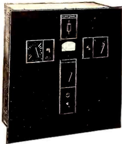
The program amplifier is a variable loss network inserted in your program circuit. The loss introduced is controlled directly by the program level.
