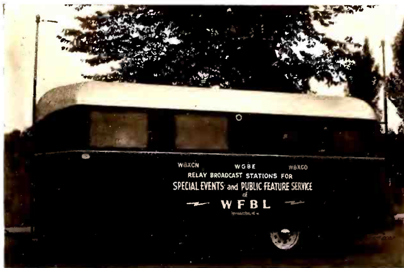
TRAIL BLAZER —WFB L, Syracuse, has equipped this trailer, easily attachable to any auto, to carry its three shortwave transmitters for special events and public address purposes at big gatherings.
