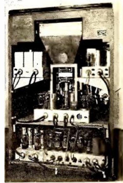
THE TELEVISION RECEIVER —At left is the console cabinet for sight and sound reception, showing the mirrored cathode-ray screen in vertical position. At right is a rear view of this experimental model of a television receiver, showing the highly complex structure with its 36 tubes. The cathode-ray projecting tube, in which bombardments of electrons "paint" the picture in black and white on the screen, is pear-shaped and stands upright within the shielding at the top. Its oval end is 12 inches in diameter, on which 9½ x 7½ in. pictures are framed.
