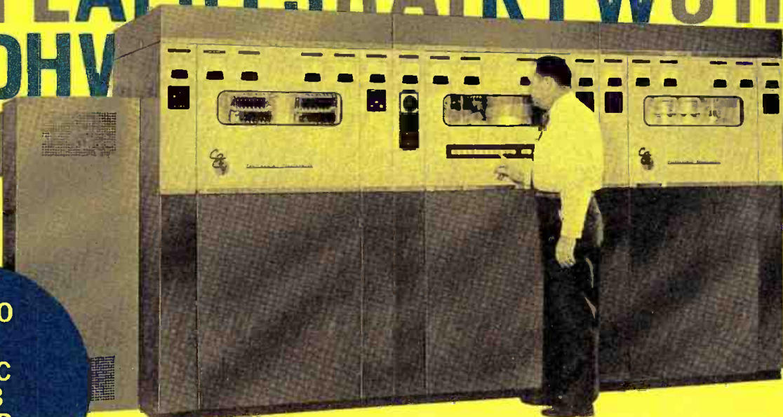
Continental Electronics Type 317C 50 KW AM Broadcast Transmitter Most popular 50,000 watt in the world.
