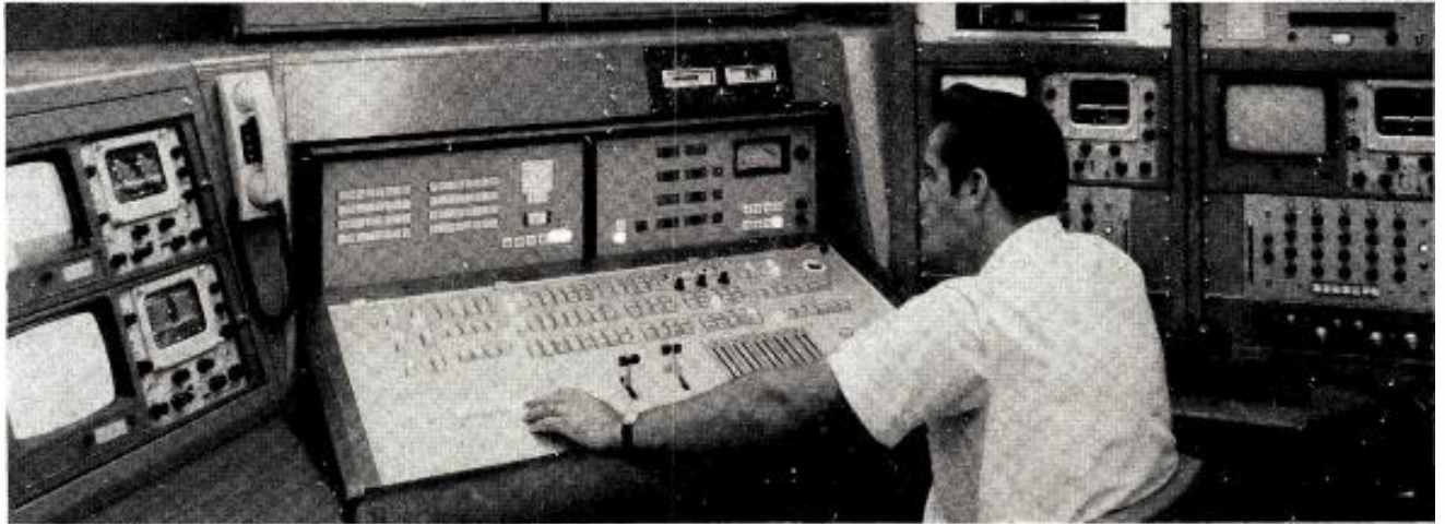
Control room at WVNY-TV, Burlington, Vt. showing CD Master Program Control System.
