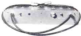
1950 First wide band distributed main line amplifier.
