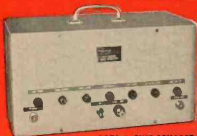
1073-A SINE-SQUARED SQUARE WAVE GENERATOR
