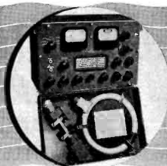
14. FIELD INTENSITY METER — The RCA, 308-A Broadcast Field Intensity Meter, designed for field or mobile use, is the standard measuring instrument used by most consultants and station engineers.
