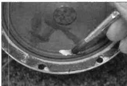
Applying Elmer's glue with a small artists brush to a tear in the cone.
