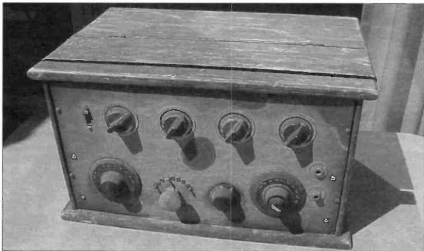
The very first Timmerman-Greene "Special" receiver, as found, unrestored by the present owner. Note that the top lid has hinges halfway back so that the cover can either be opened part way to view the tubes, or so the whole top can be opened to get at the batteries.
