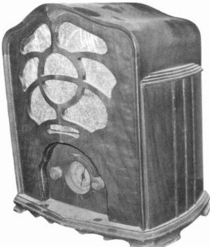
Emerson model 49 radio – A rare table radio made in 1934. Covers the BC and SW bands. Uses six tubes. Mike Katz, Seaford, NY
