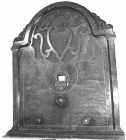
Howard model 20 radio – This cathedral radio was made in 1931. It contains seven tubes and covers the BC band. Mike Katz, Seaford, NY
