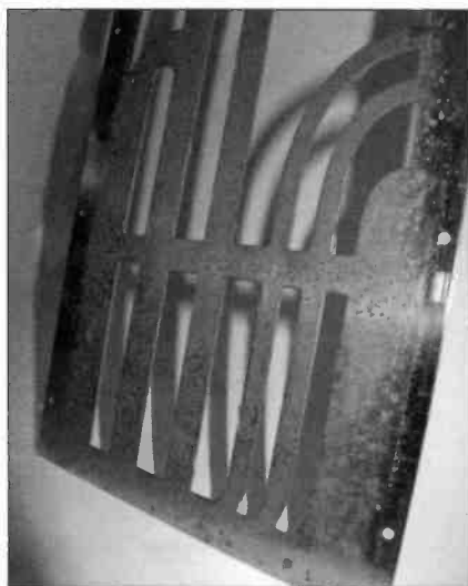
The chrome front grille removed from the cabinet and before re-chroming. Refinishing this made a huge difference in the end result.
