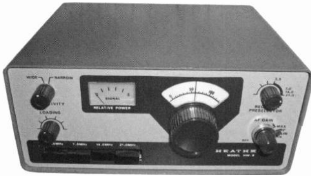
Heathkit model HW-8 transceiver – This is a QRP (low output) transceiver made by Heathkit. Came in kit form. Covers 40, 20, and 15 meters. Output approximately 7 watts. Dan Mulholland, Boise, ID
