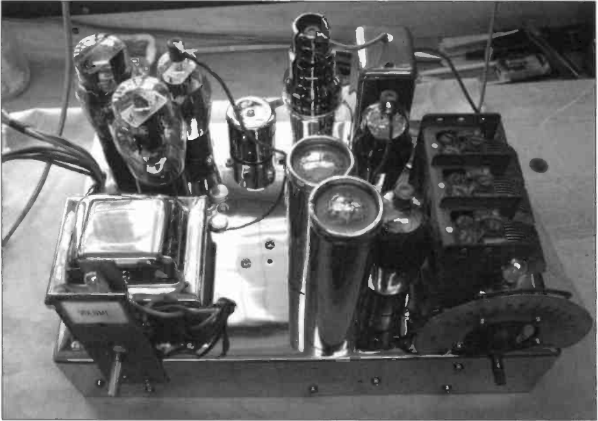
Majestic 460 chassis after chrome plating, polishing aluminum parts, and full reassembly. Dial scale is original.
