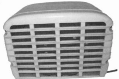
General Electric model H610-U – Manufactured in brown, ivory, and onyx "beetle" plastic colors. Has four pushbuttons and seven tubes. AM band only. Gordon Stevenson, Lawton, OK
