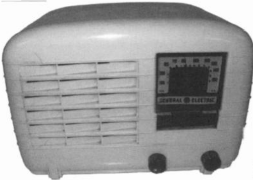
General Electric model H610-U – Manufactured in brown, ivory, and onyx "beetle" plastic colors. Has four pushbuttons and seven tubes. AM band only. Gordon Stevenson, Lawton, OK
