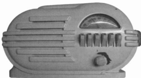
Belmont model 6D111 —This 6 tube radio was manufactured in 1946. Streamline shape with 6 pushbuttons. Ralph Brandes, Framingham, MA.
