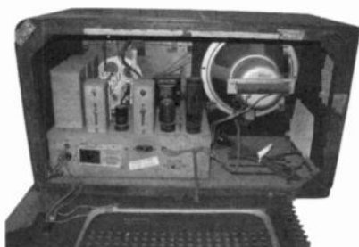
Pilot model 173 —Manufactured in 1941. Large table top radio that covers 3 bands – AM and 2 short wave. John Hewlett, Little Rock, AR.
