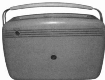
Bush Portable Radio —Model number unknown. This is an English transistor radio that works on a PP9 9 volt battery. Covers medium and longwave bands. Irwin Strongwater, Houston, TX
