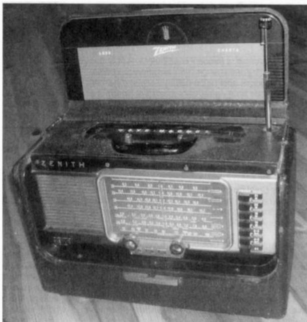
Figure 1. A typical Zenith Trans-Oceanic, a Model L-600. The L-600 followed the Models G500 and H500 and was an improved version.
