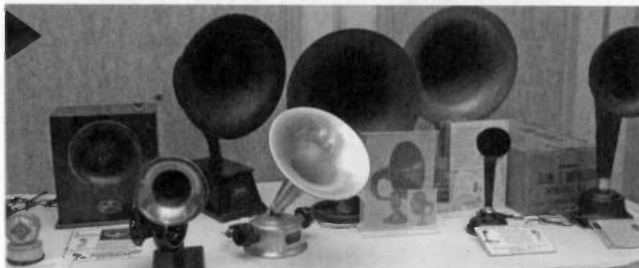
The Moon speaker, center foreground, is just a horn and uses a headset as the speaker's driver.
