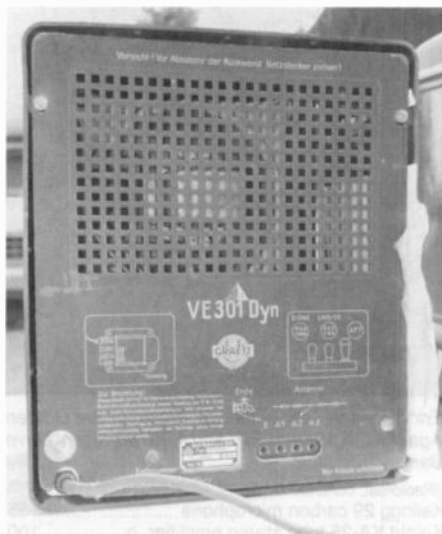
A rear view of the Graetz radio. Note the symbols for antenna and ground ("E" for erde or earth) on the rear cover.
