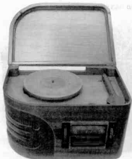
Figure 3. Nell Robar's GE Model HJ-618-AC with its lid open revealing the 78 rpm turntable and tone arm.
