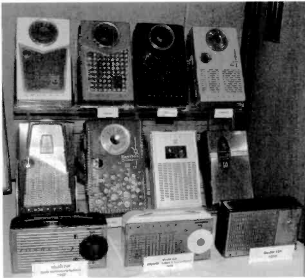
Emerson made the move from vacuum tubes to transistors, as this display of Emerson transistor radios attests. The three sets on the bottom row are the 1953 Model 747, using subminiature tubes; the 1956 Model 838, using both tubes and transistors; and the 1959 Model 555, using only transistors. The other sets above are all-transistor sets.
