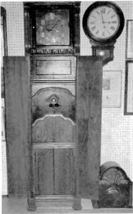
Another and very different grandfather clock radio. This 7-foot tall set, produced by the Kemper Radio Laboratories, includes a phonograph and record storage.
