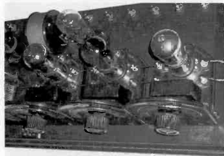
This contest entry resembles an Atwater Kent breadboard. It was manufactured by the Radio Products Manufacturing Company, RPM. Like the Atwater Kent sets, it also has individual "islands" that are mounted on a breadboard.
