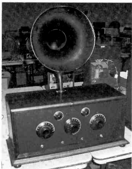
This Murdock 200 is a 5-tube Neurodyne and includes a horn speaker coming out of the top — an unusual position.
