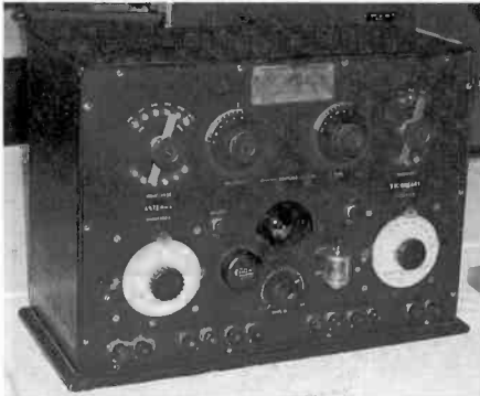
This very unusual set in the contest has a DeForest brass tag Audion, ultra-Audion, multiwave tuner with a crystal detector. If anyone out there is familiar with this unit, please contact George Potter.
