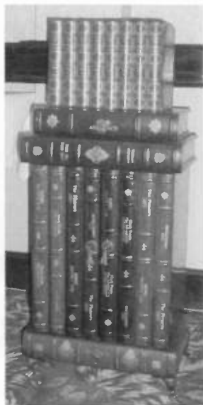
The Emerson "Library" set, ca. 1939, consists of a conventional 5-tube AC/DC chassis in a simulated leather cabinet representing several book spines. Jayne Kaiser displayed the set in the old equipment contest as shown on the right on a contemporary cabinet of similar style.
