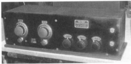
This 1922 Mu-Rad MA-13 is a 6-tube TRF set and sold for $460 without tubes.
