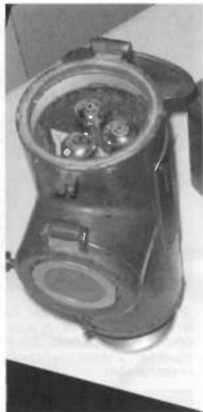
On display in the Old Equipment Contest room were three microphones from Bob Paquette's collection. The microphone with the NBC lettering is an RCA 3-A condenser microphone. The 3-tube amplifier inside is shown in the right photo. The microphone in the center is a Western Electric double-button carbon in a 1-A housing. On the right is a Western Electric 370W microphone on a D-80513 preamplifier case.
