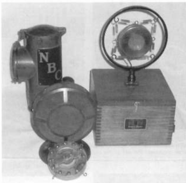
On display in the Old Equipment Contest room were three microphones from Bob Paquette's collection. The microphone with the NBC lettering is an RCA 3-A condenser microphone. The 3-tube amplifier inside is shown in the right photo. The microphone in the center is a Western Electric double-button carbon in a 1-A housing. On the right is a Western Electric 370W microphone on a D-80513 preamplifier case.
