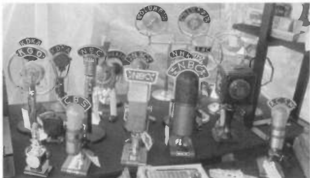
Ekkehart Willms displayed his microphones in the flea market. On the left is a Westinghouse "Tomato Can" PR-184. The array of microphones on the right were for sale. The "box" microphone is an RCA 4AA condenser microphone with amplifier. The station letter flags were reproductions.
