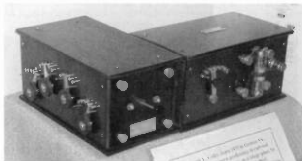
Bob Slagle entered this Colby Telegraph School tuner and detector in the Old Equipment Contest. The knob on the end of the left unit is moved in and out to change the inductive coupling.
