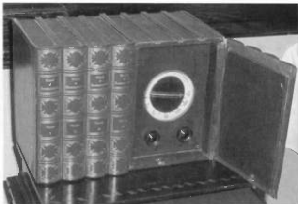
The Emerson "Library" set, ca. 1939, consists of a conventional 5-tube AC/DC chassis in a simulated leather cabinet representing several book spines. Jayne Kaiser displayed the set in the old equipment contest as shown on the right on a contemporary cabinet of similar style.
