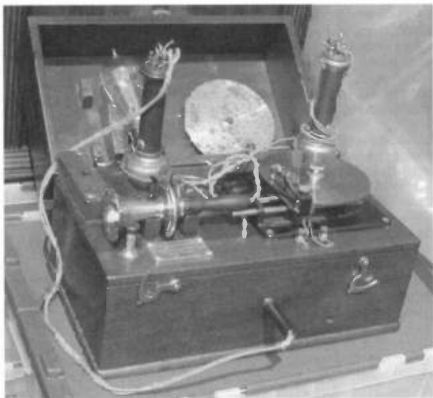
Ekkehart Wülms displayed this rare German magnetic disk recorder on his flea market table.
