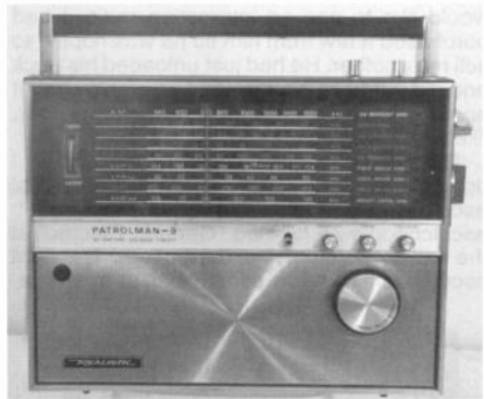
Figure 10. The Patrolman 9 has a taller case to accommodate its 9-band dial scale.
