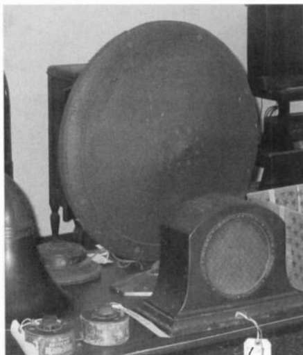
An RCA 100-A speaker is seen in front of a Western Electric cone speaker.
