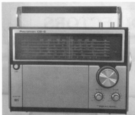
Figure 4. The Patrolman CB-6, introduced in 1978, substituted the Citizens band for the Air band.
