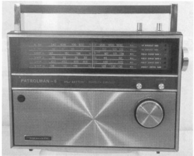
Figure 1. The first in the series of Patrolman 6 radios was this 12-756 from 1973. In addition to AM and FM, this radio tuned the High and Low VHF bands, the VHF Air band, and UHF (450-470 MHz).
