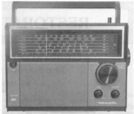
Figure 9. The DX-66, a 6-band radio, provided SW coverage. Its styling is similar to the other multiband radios described in this article.
