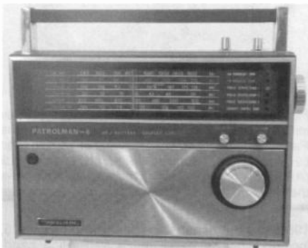
Figure 2. This Patrolman 6, a 12-760 from 1976, was identical in appearance to the 12-756. However, its UHF tuning range was extended to 512 MHz.
