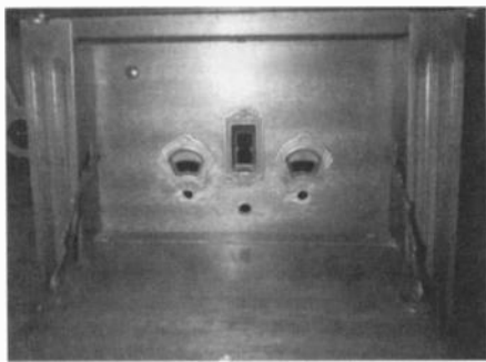
Figure 1. A front view of the radio showing the three escutcheons. The center escutcheon is the original GM item. The others are for the replacement chassis from a GE Model K-60.
