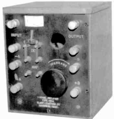
CLAPP-EASTHAM TYPE HRA – This tiny, 1-tube, 1-stage amplifier was manufactured by the Clapp-Eastham Co. of Cambridge, Mass., in 1921 to match the Clapp-Eastham Type HR 1-tube receiver. It measures 4 3 / 4 " wide by 6" high. (Wally Worth – Wollaston, MA)
