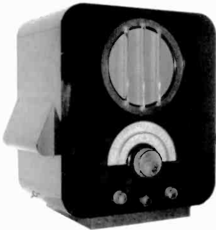
EKCO MODEL ADT95 – E.K. Cole, Ltd., Essex, England, manufactured this 7-tube radio in a black Bakelite cabinet with chrome trim and 3 vertical glass rods. It has 2 internal loop antennas and weighs about 35 pounds, which explains the side handles. (Jim Taylor – Bournemouth, England)
