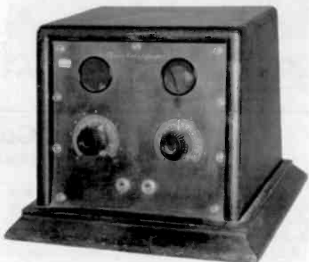
ZENITH 2-M AMPLIFIER – Manufactured by the Chicago Radio Laboratory, this 2-tube amplifier was sold to be used with the matching Zenith 1-R, 3-R, and 4-R receivers. It has the hard rubber panel with pot metal pointer dials and measures 11 \frac{3}{4} " wide x 10" tall. ( Wally Worth – Wollaston, MA )
