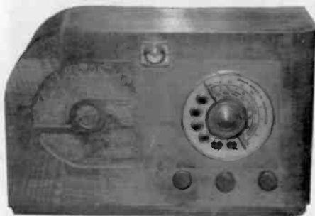
MIDWEST MODEL 11-10 OR 10-38 – The Midwest Radio Co. of Cincinnati, Ohio, manufactured this 8-tube receiver in 1938. One of the tubes is the eye tube shown at the top center of the wood cabinet. AC operated, it tunes both broadcast and shortwave bands. ( Michael G. Comer – Haslett, MI )
