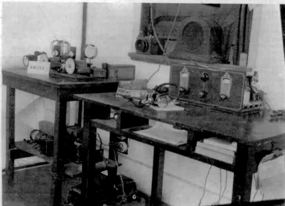
Figure 1. This Ham station, OM2CS, located on Guam, uses a factory-built receiver, a Pilot Super Wasp, and a home-brew CW transmitter.
