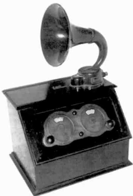
MARCONI TYPE 23 – This 2-tube receiver, manufactured in 1928, has coils moulded into the Bakelite panel. The horn speaker on top is a 1925 S.G. Brown Type H4. (Jim Taylor – Bournemouth, England)
