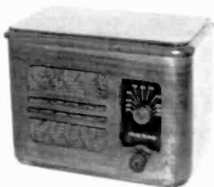
AIR KING MODEL 1001 – This all-wood, midget table radio was made in 1937. It uses the following tubes: (1) Type 6D6; (1) Type 6C6; (1) Type 43; and (1) Type 25Z5. (Clark Trissell – Lincoln, NE)
