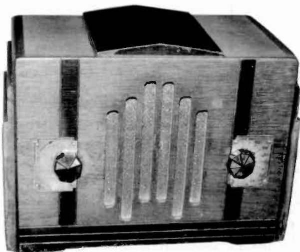
Figure 1. This small 4-tube AC/DC TRF radio of the mid-1930s lacks a manufacturer's name.
