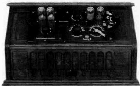
RCA RADIOLA III – This Radiola III is set in an original ACRE Deluxe cabinet, which includes the 2-tube RCA balanced amplifier and built-in speaker below. The radio operates on (4) Type WD-11 tubes, but could use Type UX-199 or Type 230 tubes with WD-11 adapters. When these substitute tubes are used, the knob at the bottom of the grille controls the filament current. ( Ross Mason – Mason City, IA )
