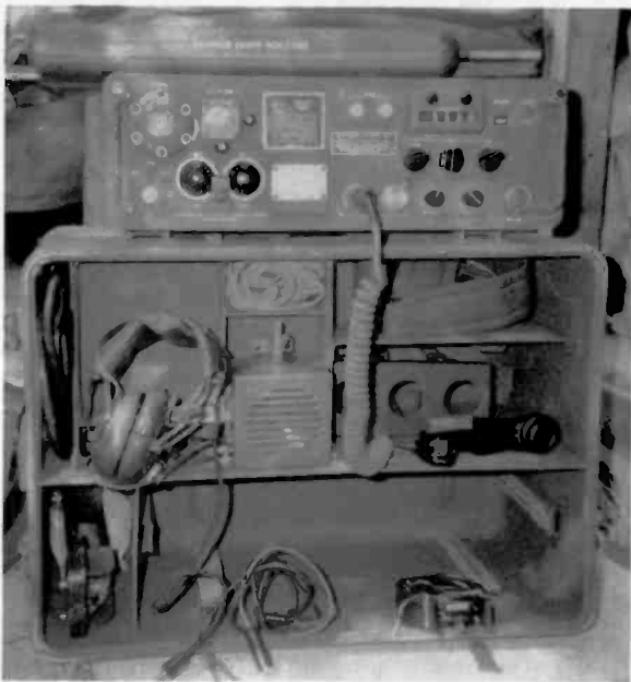
The AN/PRC-47 sitting on top of its carrying case, which also has provisions for storing accessories.
