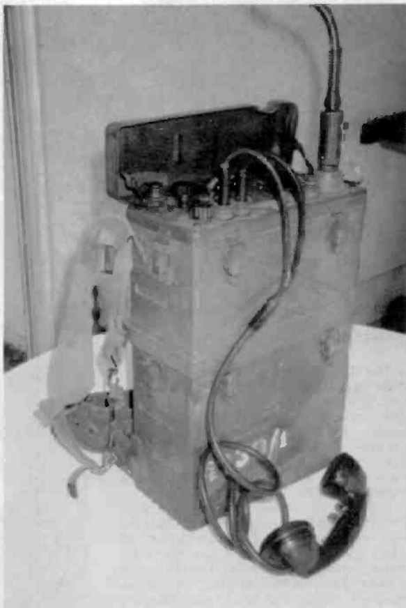
The SCR-300-A is shown with the antenna attached, the handset plugged into the set, and the battery box on the bottom. Carrying straps for backpack operation are attached.
