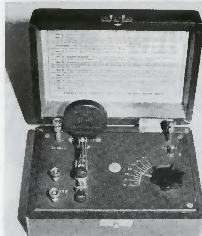
Figure 4. The long-wave coil in place at the top left of panel.
