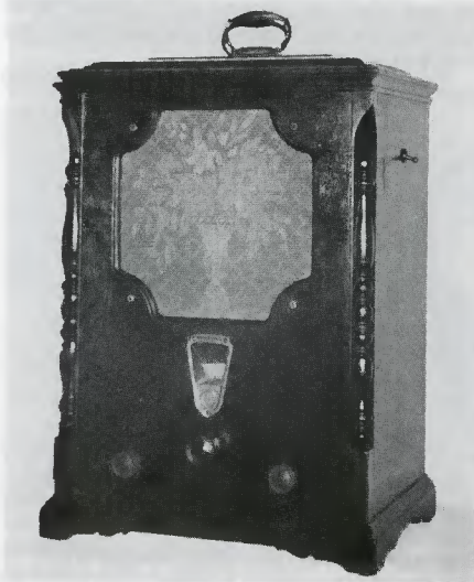
Figure 1. The GE Model S-22's unusual features are the brass handle and the open grille cloth area.
