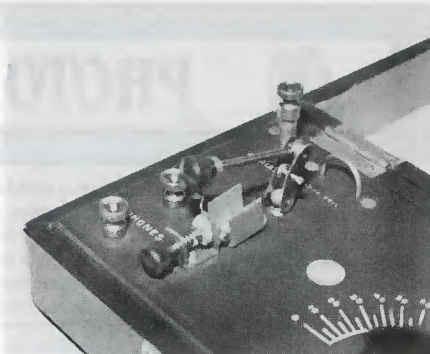
Figure 5. Close-up of the detector showing rear-pivoted detector arm and crystal holder with cover.
