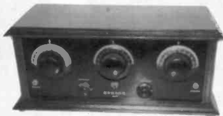
ADROLA MODEL R5P – This 1925 TRF battery set is a rare model from the Adroit Tool Co. Five Type 201-As are behind the front Bakelite panel in a neat symmetrical layout. Three tuning condensers are employed with Freshman-style coils. Two audio transformers are used in the AF stages. Please contact A.R.C. if you have any information concerning the Adrola series of radios. ( Orval Egarter – Fonthill, Ontario, Canada )
