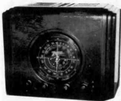
ZENITH MODEL 5S126 – This is an early example of the Zenith big black dial radios of the 1930s. It features a 5-tube, transformer-powered chassis, split-second tuning, and a top-mounted speaker providing unidirectional sound. It was manufactured in 1936 and is often referred to as one of the "cube" radios. ( William Dalton, Jr. – Bridgeport, CT )
