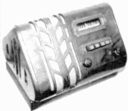
STEWART-WARNER MODEL 91-513 – This table radio, ca. 1938, has a wooden triangular case with cutouts on all 4 sides. The end view resembles a spade in a deck of cards. It features a slide-rule dial, 4 pushbuttons, and a 5-tube chassis. It is in original mint condition and plays well. Has anyone else seen one like it? (Mr. & Mrs. L. M. Page – Mullins, SC)
