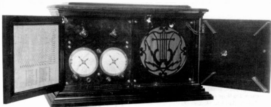
An RCA photograph taken July 20, 1923, appearing to be the Radiola XI — The Jewel. The table designed for it is not shown here. (From the Alan Douglas collection of Arthur F. Van Dyck photos.)
