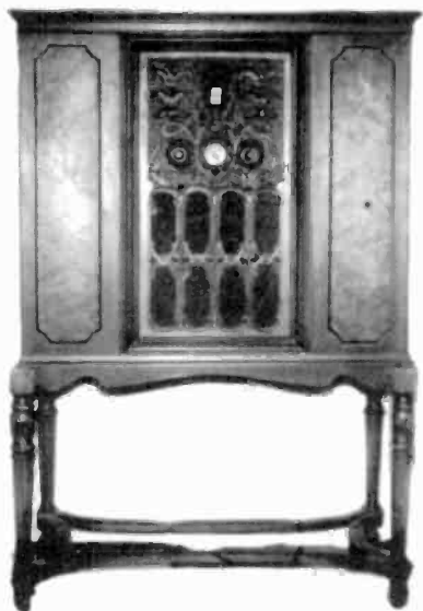
EVEREADY MODEL 42 – This 8-tube AC console, produced in 1929, has the same cabinet and chassis as the Model 32, except for the use of Type 45 output tubes. The cabinet has very decorative Repwood in the center section. The set originally sold for $180. (William Bourke – Swampscott, MA)
