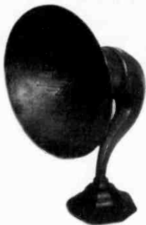
MERCURY RADIO CO., N. Y. – This horn speaker named "Grand," ca. 1925, has a heavy cast-iron base and weighs a total of 12 pounds. It has a beautiful nickeled driver and still works! (Wally Worth – Wollaston, MA)
