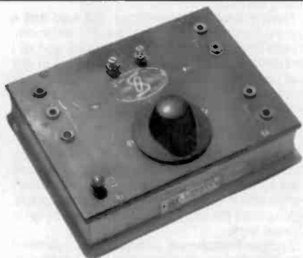
SCHNEIDER-OPEL CRYSTAL SET – This crystal set was manufactured in Frankfurt Germany by the F. Ehrenfeld Company. The detector has been missing since I acquired it in the early 1950s. Otherwise, it is complete. (Norman Hart – Clearwater, FL)
