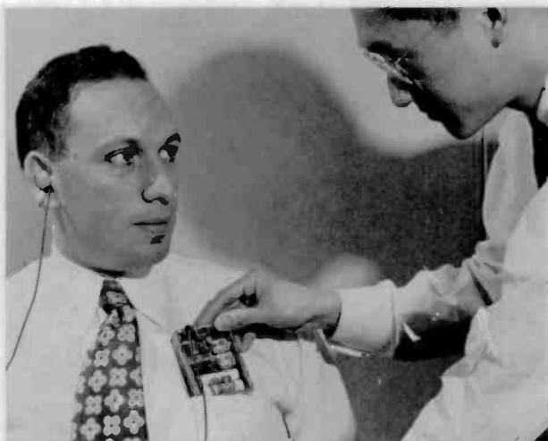
Figure 4. GE engineers in 1954 demonstrate an experimental pocket radio, designed primarily for emergency broadcast use by civil defense workers, who could wear it like a hearing aid. ("Herald Tribune" photo, from the editor's collection.)
