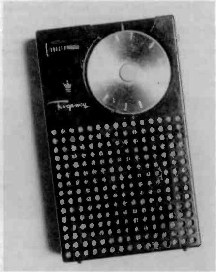
Figure 5. The Regency TR-1, the first all-transistor portable radio, manufactured by the I.D.E.A. Company in 1954. (From the George Kaczowka collection.)
