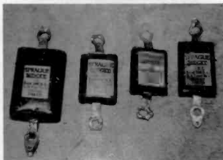
Figure 2. Early paper capacitors from Sprague. Their values, left to right, are 0.25, 0.02, 0.02 and 0.01 mF. All are rated at 400 vdc, except for the 0.01 mF, which is rated at 500 vdc. Note the flat tinned-copper, solder-lug type of leads.
