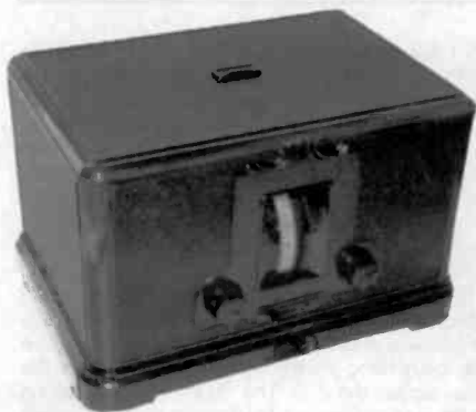
EKCO MODEL 312 – This 2-tube AC radio is of 1930 vintage. The cabinet is completely made of Bakelite material. (Jim Taylor – Winton, Bournemouth, England)
