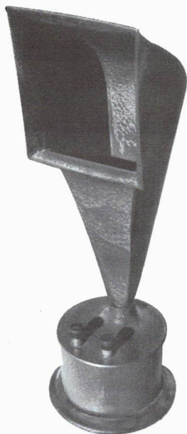
TRINITY TYPE A HORN SPEAKER – This square-shaped metal horn was manufactured by the Trinity Radio Company of Boston, Mass. The bottom of the round metal base has a turned wooden trim. The metal parts are painted a reddish mahogany color. Later versions of this speaker had a more common round shape to the bell and neck. ( Dave Crocker – Mashpee, MA )
