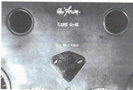
Figure 3. Closeup of the detector hole cover plate on the De Forest D-12 panel, version 3.
