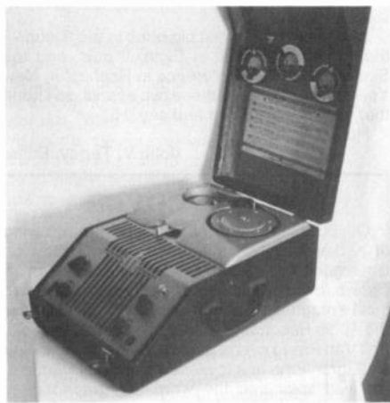
Figure 1. The Webster Chicago Model 80 single-channel, tube-type wire recorder, ca. 1947-1952, is AC-operated and uses a single motor to run the wire at 24 ips.
