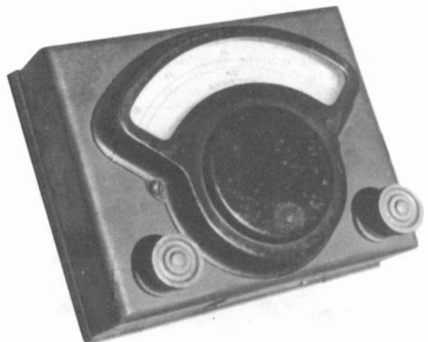
Figure 2. An AC ammeter manufactured by Hoyt about the same time as the Model 100 tube tester.
