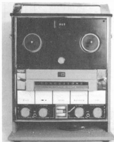
Figure 6. The Concertone Model 800 "Revers-O-Matic," ca. 1966-1967, features 6 heads and is an AC-operated hybrid. It uses 3 motors and operates at tape speeds of 7½ and 3¼ ips.
