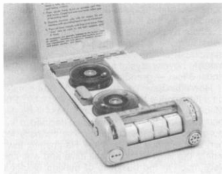
Figure 2. The transistorized, battery-operated Minifon Model 360S wire recorder, ca. 1961-1963, is a single-motor, single-channel recorder. Produced in Germany and used for surveillance, it operates at 13.4 ips.
