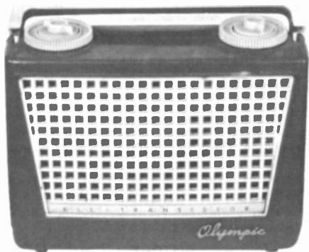
OLYMPIC MODEL 447 – This 1956 AM battery transistor radio is the size of a lunch box. The transistors were installed in tube sockets. ( Kurt Henriksen – Peotone, IL )
