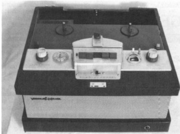
Figure 3. This 2-channel, tube-type Voice of Music tape recorder, Model 714, ca. 1955-1957, operates on AC at 7½ or 3¼ ips and accepts 7" reels.
