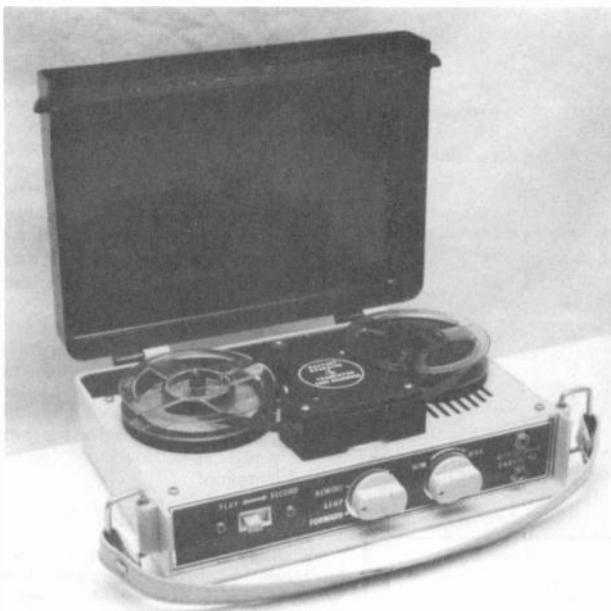
Figure 4. The single-channel Apollo Model Apolec tape recorder, ca. 1962-1964, is transistorized and battery-operated. It accepts 3" reels.
