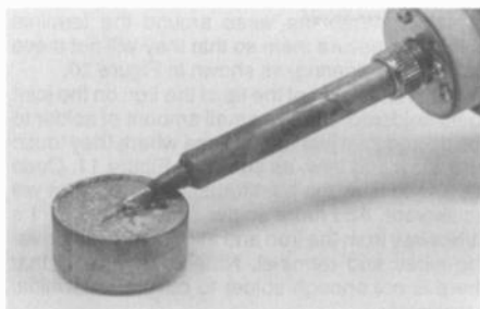
Figure 7. Using a product like the Multicore TTC1 tip tinner/cleaner makes the job easier when using volatile low residue solder.
