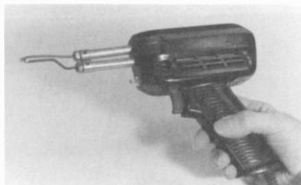
Figure 3. This Weller soldering gun is typical of those used in radio repair.
