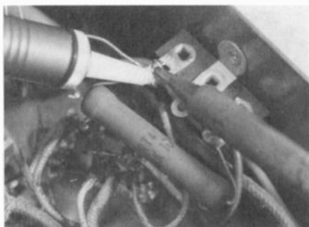
Figure 14. A solder sucker, shown at left, is a helpful tool when removing solder from a large terminal.
