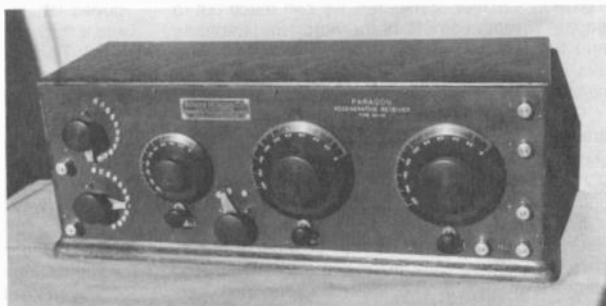
Figure 1. The Paragon RA-10 regenerative shortwave tuner.
