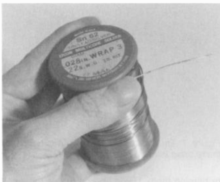
Figure 6. A 1-pound roll of 22 gauge 62/36/02 tin/lead/silver solder. The code "WRAP 3" printed on top of the roll means "wire solder with rosin activated flux in the quantity of 3 percent."
