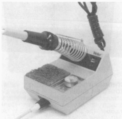
Figure 2. A Weller WTCPN soldering station with soldering iron holder. Note the sponge on the left and the TTC1 tip tinner/cleaner on the right.
