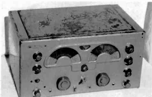
Figure 3. The badly worn finish on this National NC-173 cabinet can be compared to a bad finish on a wooden set.
