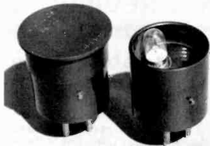
Figure 4. The tube substitute with the black plastic cap in place.
