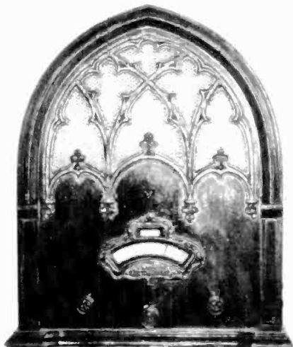
ECHOPHONE MODEL 14 – This 6-tube superheterodyne, ca. 1932, has shadowgraph tuning and tone control. Phone jacks are mounted on the rear apron. (Ed Paski – Berwyn, PA)
