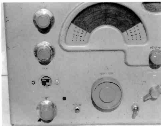
Figure 5. The original variable tone control on this National NC-173 has been replaced by a slide switch, shown at left, second from the bottom.
