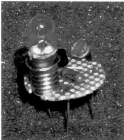
Figure 2. Tube substitution components, mounted on a circular piece of perforated board.
