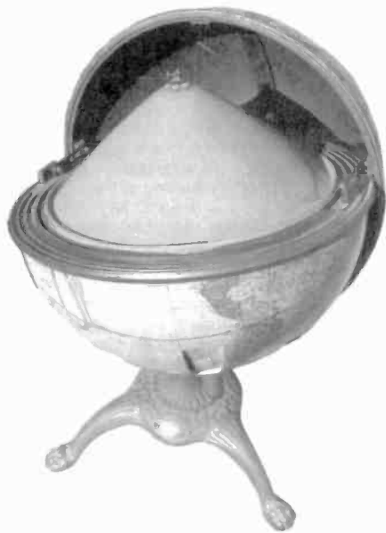
Figure 2. The Symphonic Globe speaker opened at its equator to show the cone. Also note one of the covered speaker openings on the lower section.
